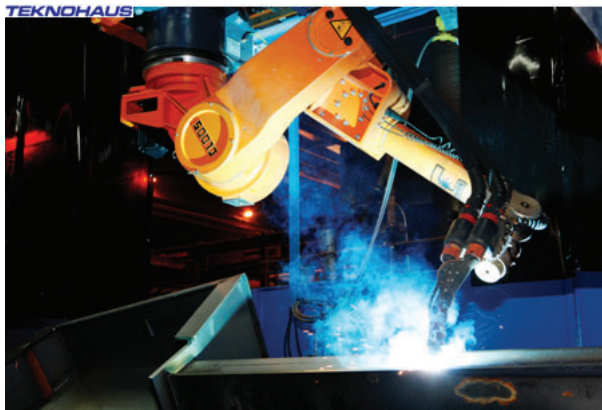
Photo. Welding the frame for a heavy-duty forest machine uses up to 45 kg of filler metal. Source: Teknohaus.
